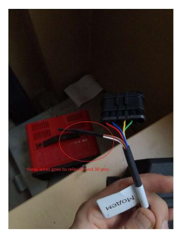
Those wires connects to "30" and "87" pins of relay
